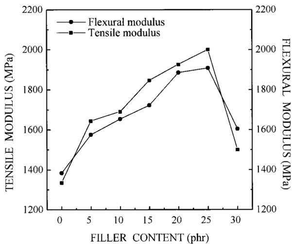
**Figure 8** Tensile modulus and flexural modulus versus filler (kaolin) content for blocked PU (15 wt %)-VE (85 wt %) IPNs.
