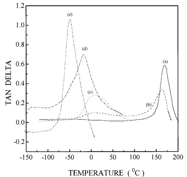
**Figure 14** Dynamic damping curve ( $\tan \delta$ ) versus temperature for blocked PU-VE IPNs at various blocked PU-VE compositions (wt %), as follows: (a) 0/100; (b) 30/70; (c) 50/50; (d) 65/35; (e) 100/0.
