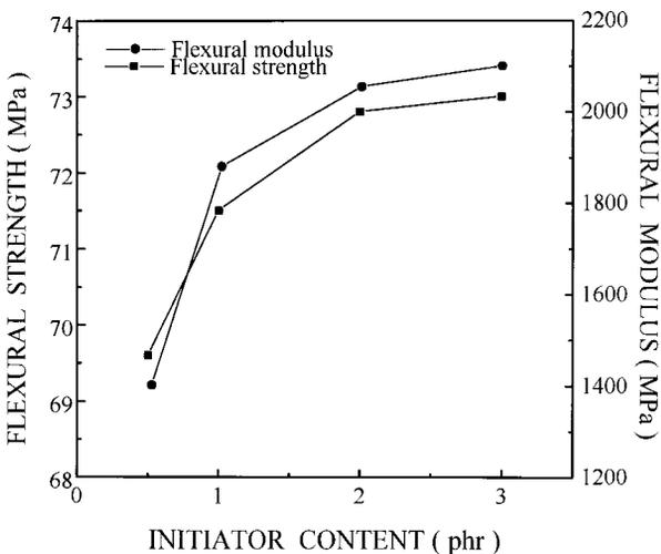
**Figure 12** Flexural strength and flexural modulus versus initiator content of VE for blocked PU (15 wt %)-VE (85 wt %) IPNs.
