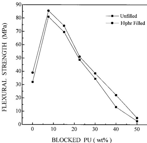
**Figure 2** Flexural strength versus blocked PU content for unfilled (—■—) and 10 phr filled (kaolin) (—●—) of blocked PU-VE IPNs.
