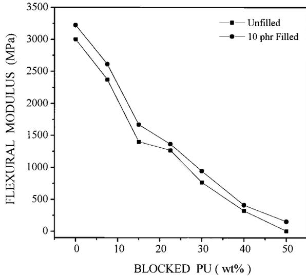
**Figure 4** Flexural modulus versus blocked PU content for unfilled (—■—) and 10 phr filled (kaolin) (—●—) of blocked PU-VE IPNs.
