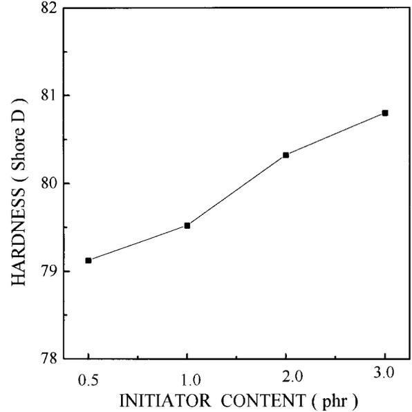
**Figure 13** Shore D hardness versus initiator content of VE for blocked PU (15 wt %)-VE (85 wt %) IPNs.
