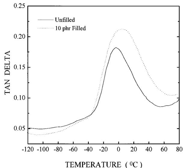
**Figure 16** Dynamic damping curve ( $\tan \delta$ ) versus temperature for unfilled (—) and 10 phr filled (kaolin) (···) of blocked PU (40 wt %)-VE (60 wt %) IPNs.
