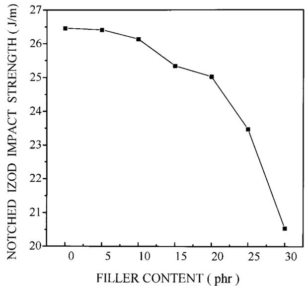
**Figure 10** Notched Izod impact strength versus filler (kaolin) content for blocked PU (15 wt %)-VE (85 wt %) IPNs.
