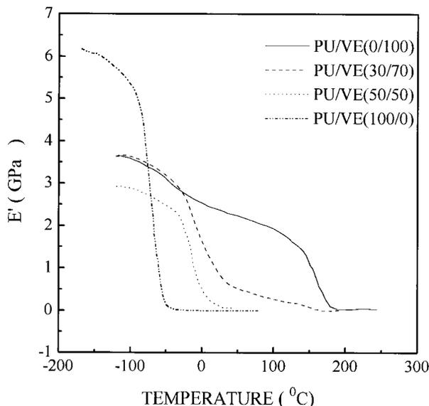
**Figure 15** Dynamic storage modulus ( $E'$ ) versus temperature for blocked PU-VE IPNs at various blocked PU-VE compositions (wt %).
