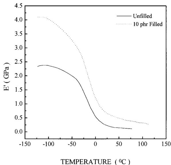
**Figure 17** Dynamic storage modulus ( $E'$ ) versus temperature for unfilled (—) and 10 phr filled (kaolin) (···) of blocked PU (40 wt %)-VE (60 wt %) IPNs.
