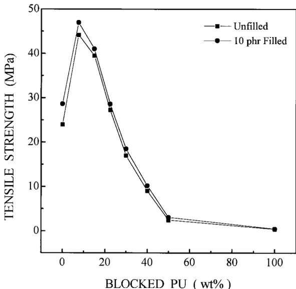
**Figure 1** Tensile strength versus blocked PU content for unfilled (—■—) and 10 phr filled (kaolin) (—●—) of blocked PU-VE IPNs.
