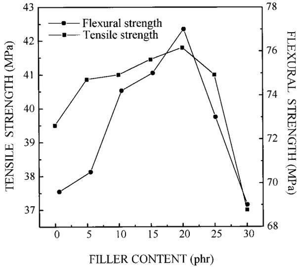
**Figure 7** Tensile strength and flexural strength versus filler (kaolin) content for blocked PU (15 wt %)-VE (85 wt %) IPNs.
