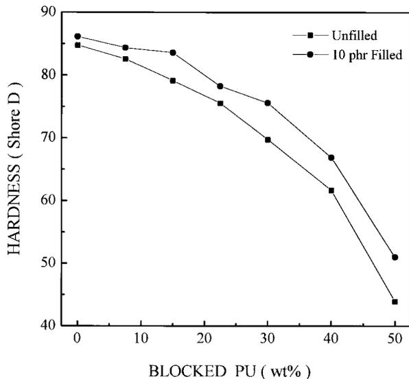
**Figure 5** Shore D hardness versus blocked PU content for unfilled (—■—) and 10 phr filled (kaolin) (—●—) of blocked PU-VE IPNs.
