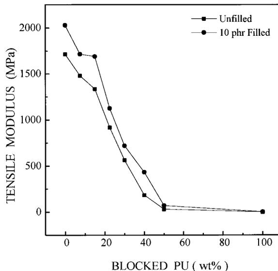
**Figure 3** Tensile modulus versus blocked PU content for unfilled (—■—) and 10 phr filled (kaolin) (—●—) of blocked PU-VE IPNs.
