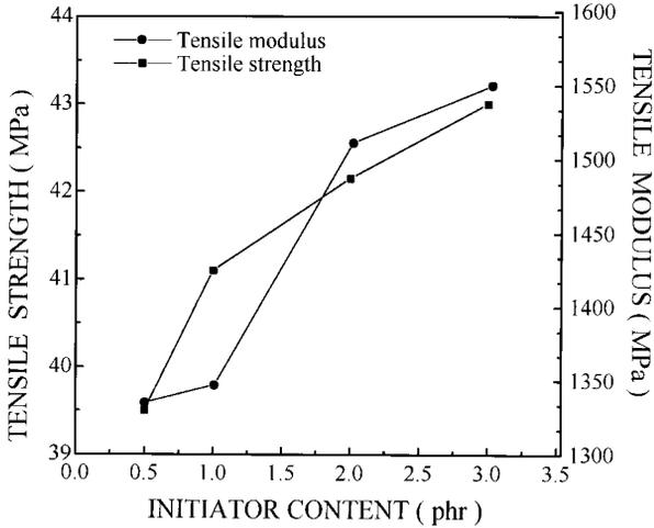
**Figure 11** Tensile strength and tensile modulus versus initiator content of VE for blocked PU (15 wt %)-VE (85 wt %) IPNs.
