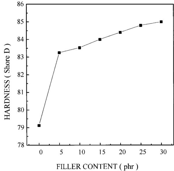
**Figure 9** Shore D hardness versus filler (kaolin) content for blocked PU (15 wt %)-VE (85 wt %) IPNs.
