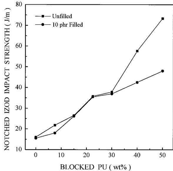
**Figure 6** Notched Izod impact strength versus blocked PU content for unfilled (—■—) and 10 phr filled (kaolin) (—●—) of blocked PU-VE IPNs.
